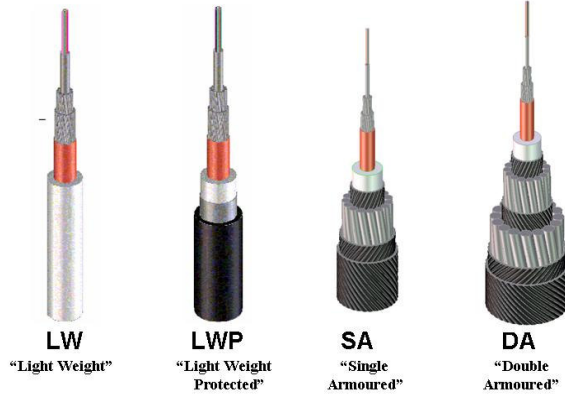
Figure 29: Sections of the undersea cable.
